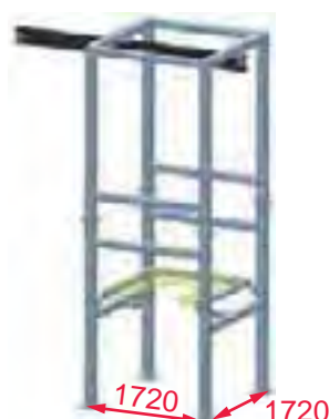
Fig.: Cantilever gantry with runway girder and support table
