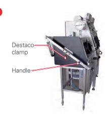
Open the Destaco clamp and lift door 1 using the black handle Push a sack onto the roller conveyor in the feeding lock.
