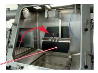
Use the gloves to pull the sack into the glovebox. 6
