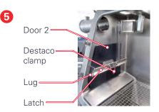
Reach into the gloves and open the Destaco clamps.
