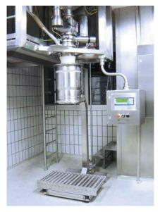
The HECHT Spoon Sampler is a convenient inline sampling system with a flexible sampling vessel (spoon) that can be operated either pneumatically or manually.
