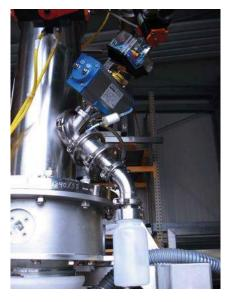
The HECHT Vacuum Sampler is ideally suited for closed and automated inline-sampling of powders and granulated materials from a product column.
