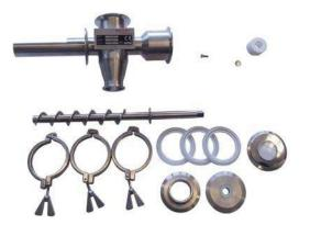
The sampling screw rotates into the material flow, extracts a representative cross-section from the production flow and transports it into a sample vessel. An adjustable timer determines the sample quantity.
