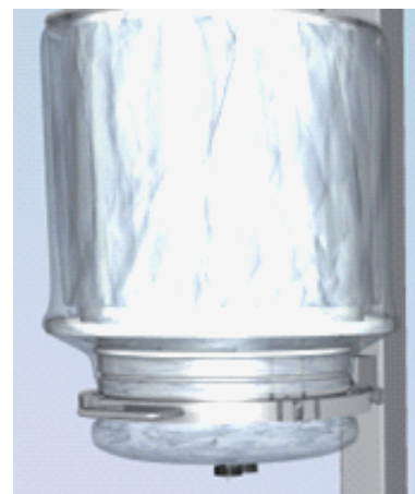
9 Cut the liner in between the two clips.
