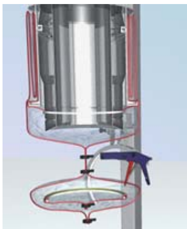
8 Remove the lower clamping ring and the old liner. Close twice.
