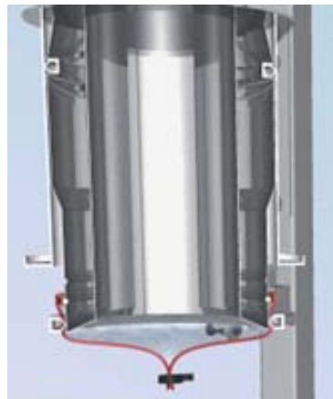
2 Move the clamping ring into the lower groove fixing the liner end.
