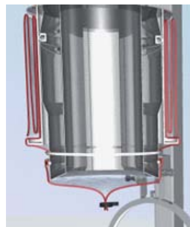
6 Fixate one end of the liner by a clamping ring in the upper groove.
