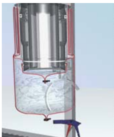
7 Pull down the other end of the liner and close it with the closing tool.
