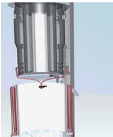
5 Put a new liner package onto the carrier.
